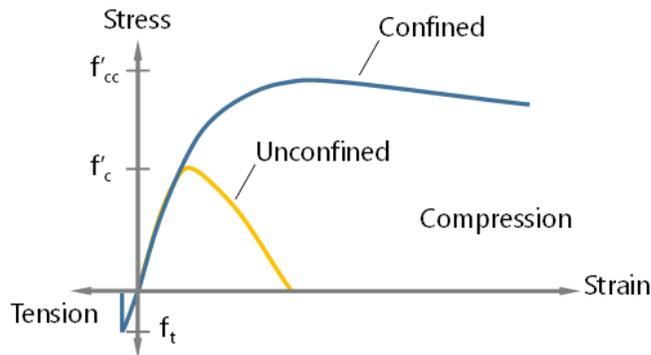
Figure 15. Stress-strain relationships for modeling of confined and unconfined portions of concrete cross-sections
