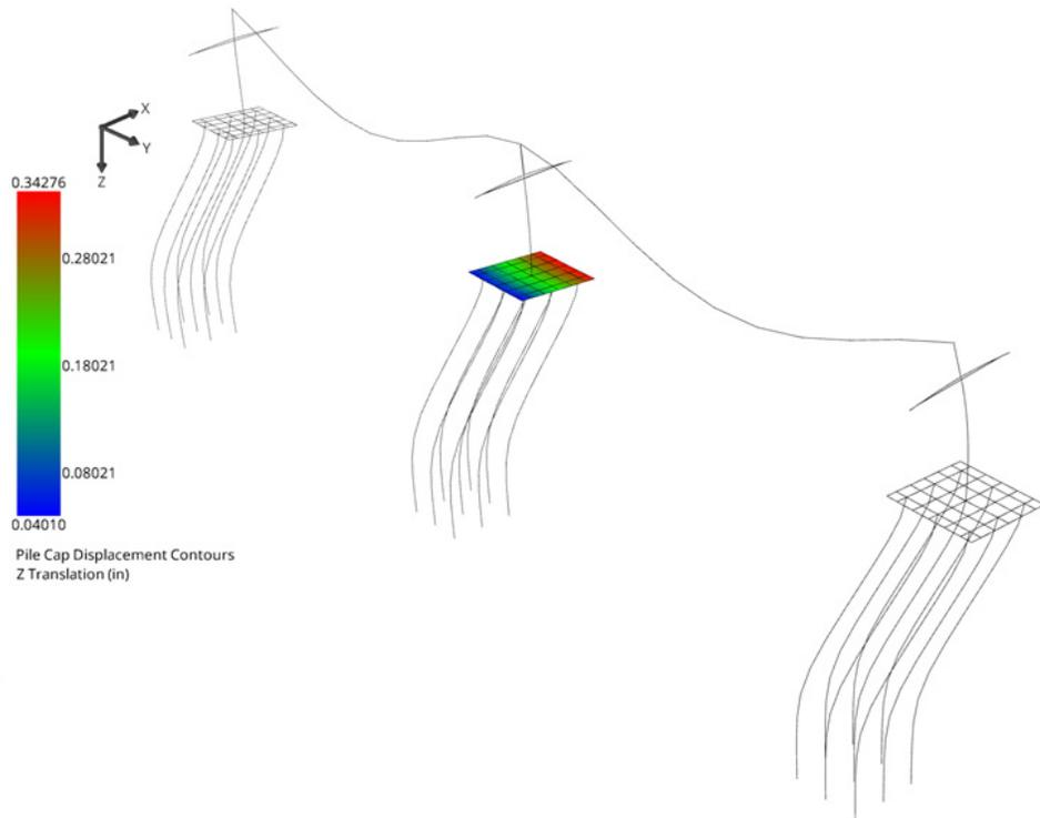
**Figure 5. Deformed structure with vertical displacement contours of the pier-2 pile cap**
