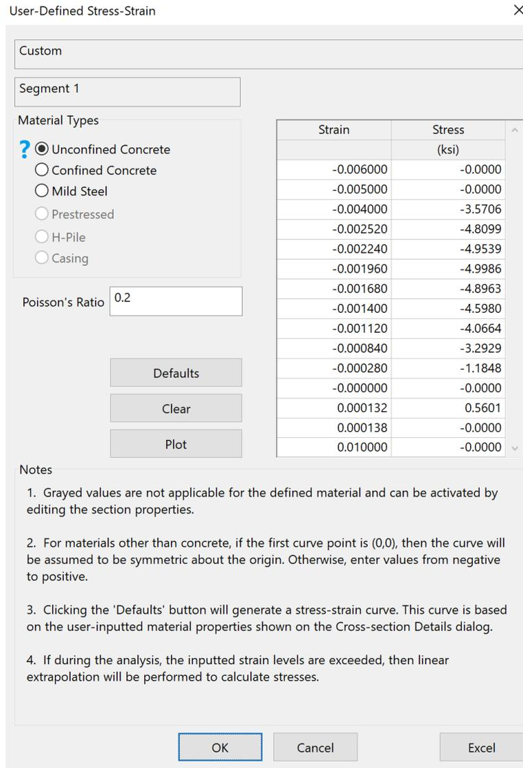
Figure 18. User-Defined Stress-Strain dialog with illustrative input for Unconfined Concrete
