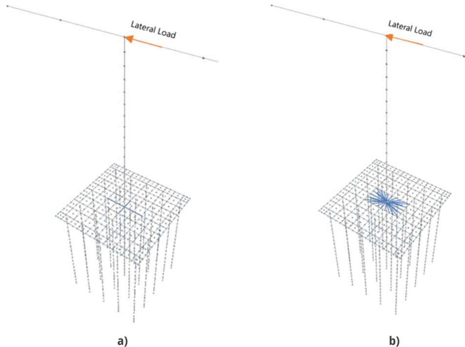
Figure 11. Model configurations: a) Quad-link approach; b) Multi-link approach
