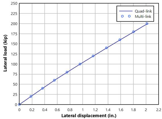
Figure 13. Lateral load v. lateral displacement at location of applied lateral load
