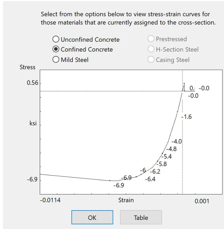
Figure 21. Stress-Strain Plot for Confined Concrete
