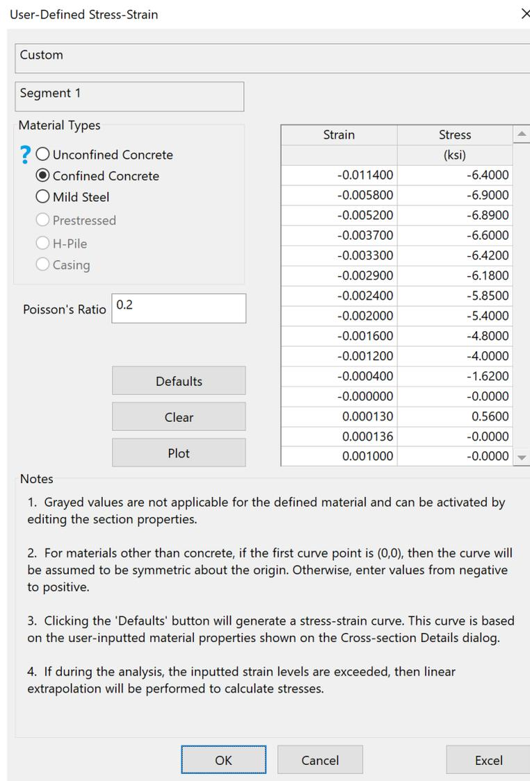
Figure 20. User-Defined Stress-Strain dialog with illustrative input for Confined Concrete
