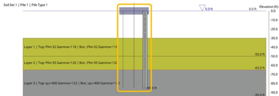
**Figure 4. Soil Edit window with selected pile, soil layering, and foundation “silhouette”**
