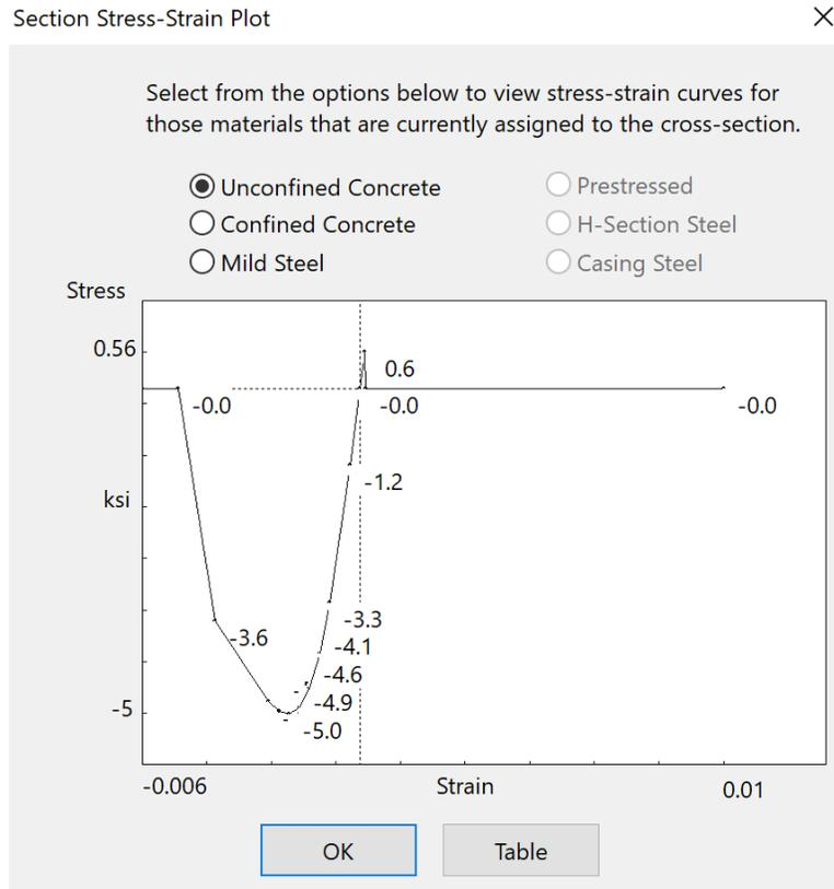
Figure 19. Stress-Strain Plot dialog for Unconfined Concrete
